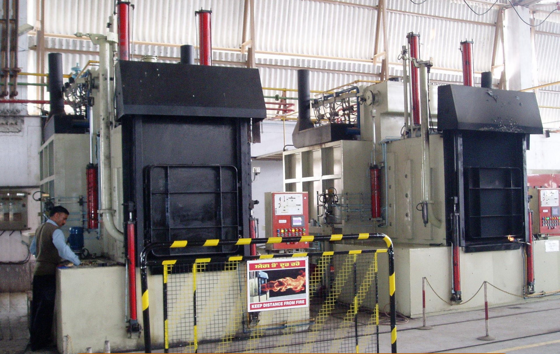
Seal Quench Furnace, GNA Duraparts, Hoshiarpur Furnace Coated with Internal & External Thermo Ceramic Coatings
